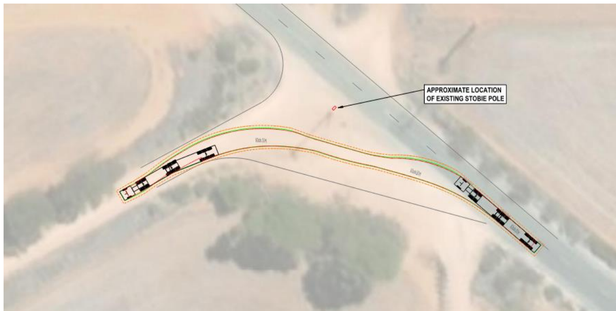
Figure 5.7: 26 metre B-Double Koolunga Rd/Power Station Road Left Turn Entry
