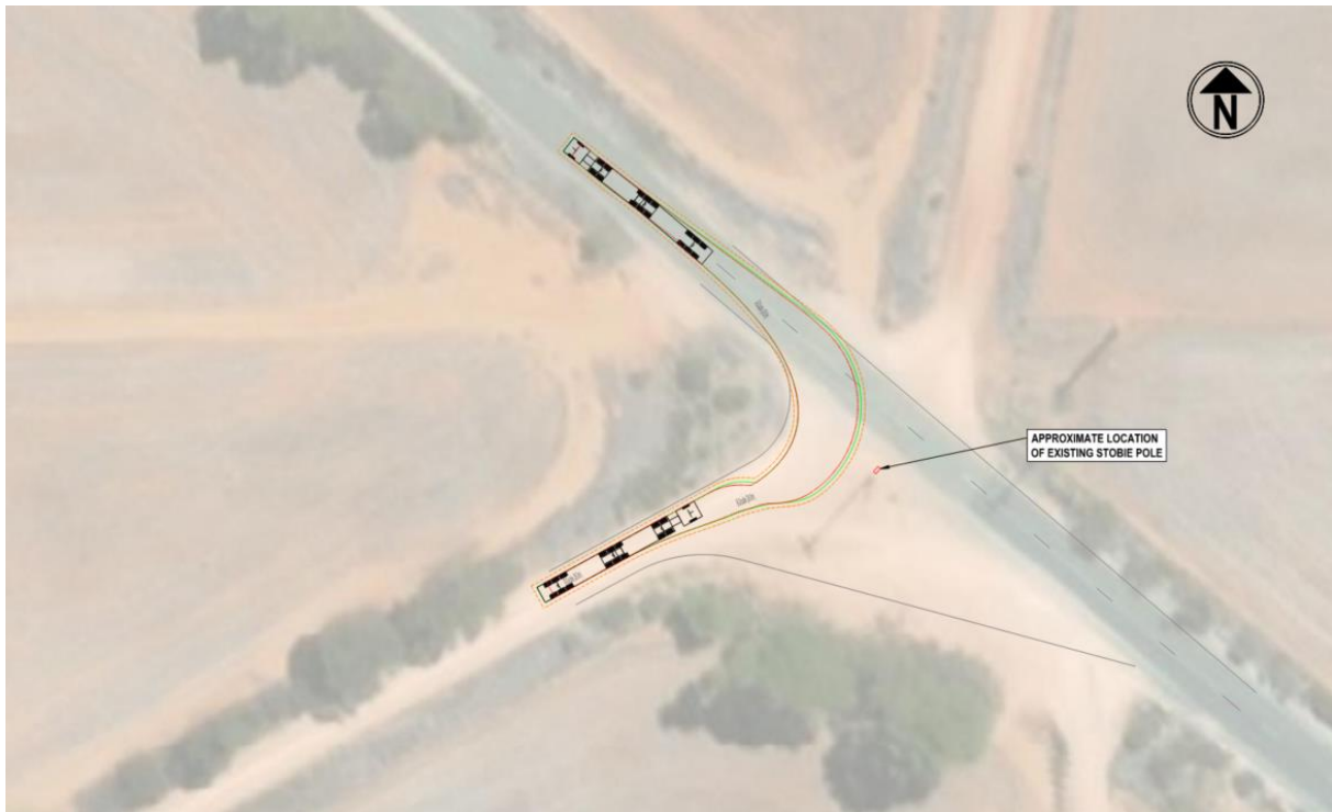
Figure 5.3: 26 metre B-Double Koolunga Rd/Power Station Rd Left Turn Exit
