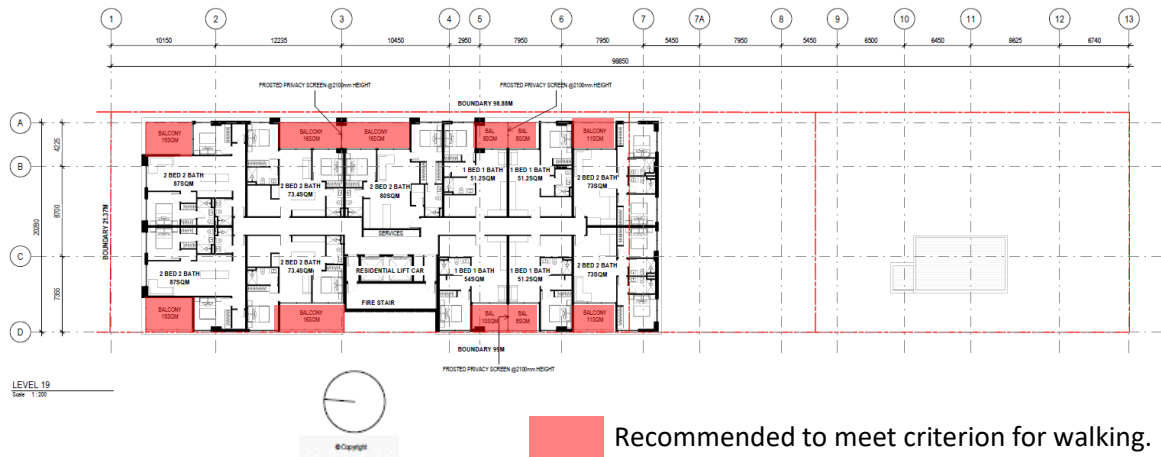
Figure 13: Schematic plan view of proposed development with recommended wind criteria overlaid on Level 19
