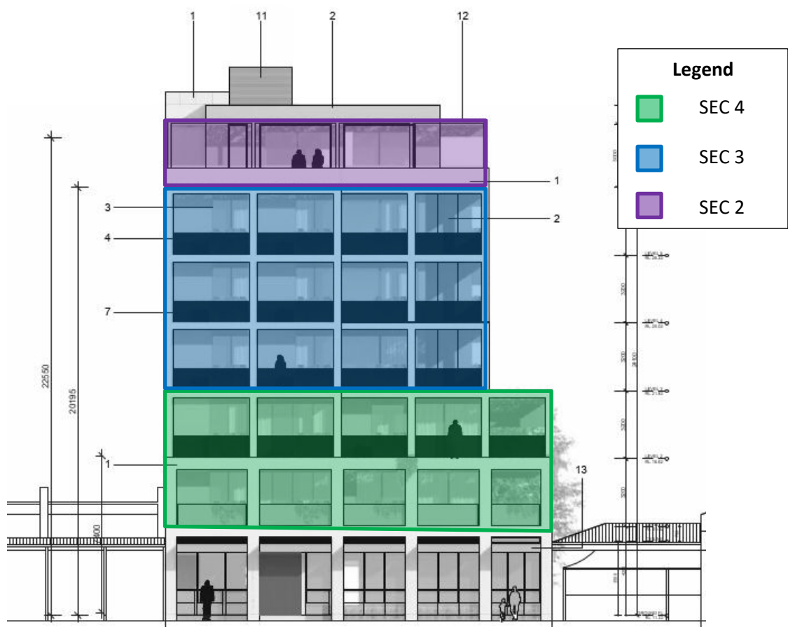
Figure 2: SECs for the eastern facades exposed to Designated Sound Sources
