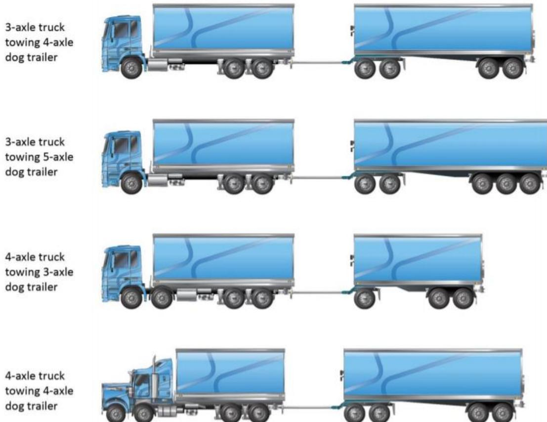
**Figure 52: Proposed truck and dog combinations** (National Heavy Vehicle Regulator - National PBS Truck and dog trailer notice Information Sheet – May 2016)
