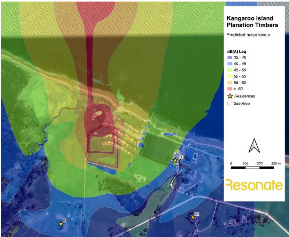
**Figure 27: Predicted noise levels (terrestrial) during operation of the proposed facility** (Response Document Appendix H Figure 1)
