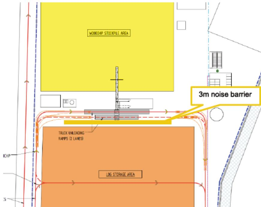
**Figure 29: Recommended (Resonate) additional noise barrier** (EIS Appendix N Figure 6)
