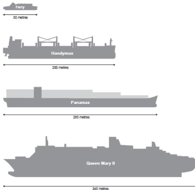
Figure 47: Comparative indication of vessel sizes (EIS Figure 21-9)
