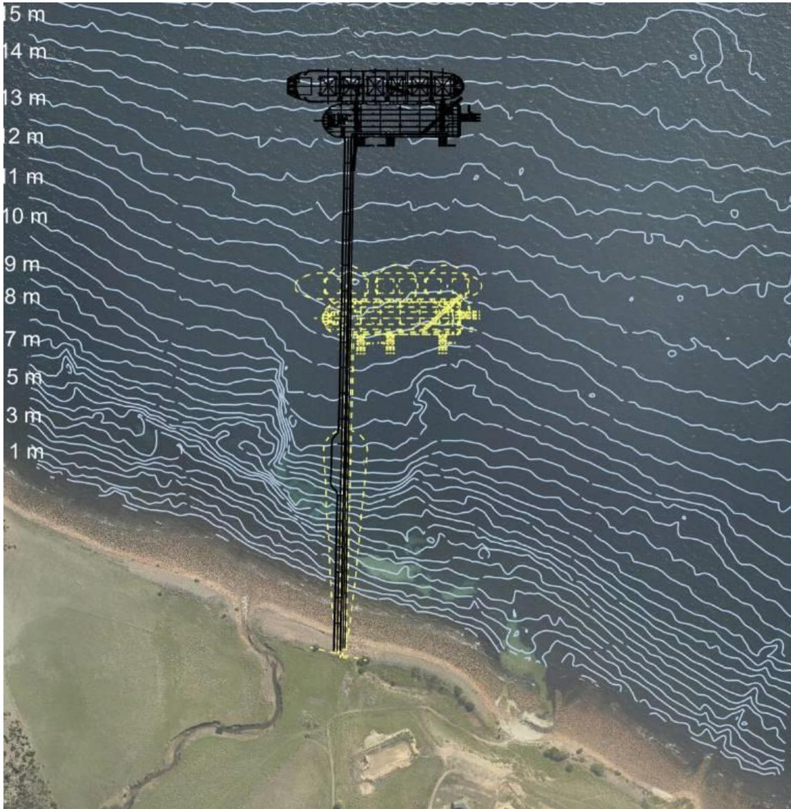
**Figure 2: Comparison of the in-water structure proposed in the EIS (yellow) with that proposed in the Addendum to the EIS (October 2019) (black)** (Addendum Figure 3-2)
