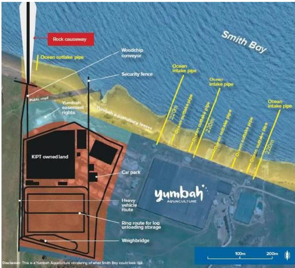
**Figure 60: Location of Yumbah’s intake pipes**
