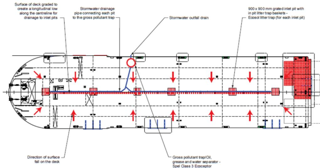
**Figure 14: Wharf/berge surface water management system** (EIS Figure 4-6)
