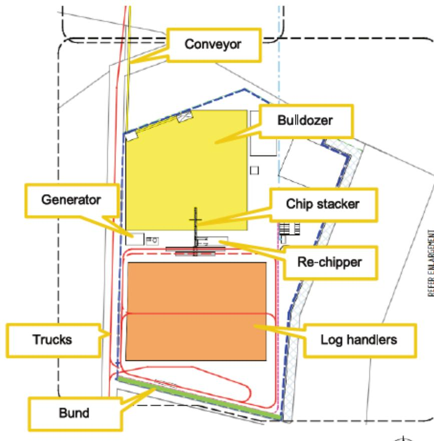
**Figure 28: Overall site layout (showing noise sources) and proposed bund along southern boundary** (note: re-chipper is no longer proposed, this component was removed after the original noise modelling was conducted) (EIS Appendix N, Figure 4)
