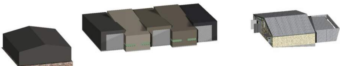
FIGURE 2. Proposed development: the proposed shed of 30m x 17m (510m 2 ), expressed as 5 modules alternating front to back, provides for greater separation from the farm building and stone barn creating a less crowded feel with the same size of building, and maintaining a sense of open space in the Depot
