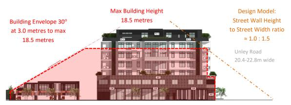
Limited rear built form and mass is positive and that the whole built form and extra tower height is contained within the fundamental zone boundary transition interface building envelope;
