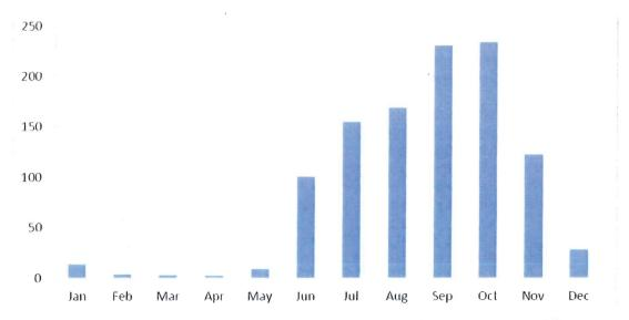
Figure 8: Average monthly volume (ML) stored at Wingate Dam, based on 1973-1995 flows
