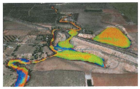
Figure 14: Wingate Dam: Up to 1 in 50 ARI floods are contained in the river channel
