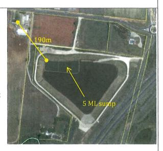
9 SA Water requires that VPS water is taken into a storage. Some customers use tanks, but the most common receptacle is an above-ground 'turkey-nest' storage. The nearby storage shown below is on Gawler River Road, and nearest sensitive receptors are 70m and 110m away.
