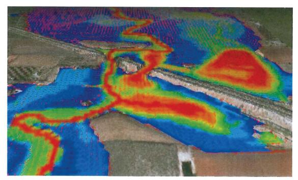
Figure 15: Wingate Dam: Events above 1 in 50 over-top the dam (1 in 100 year ARI shown)
