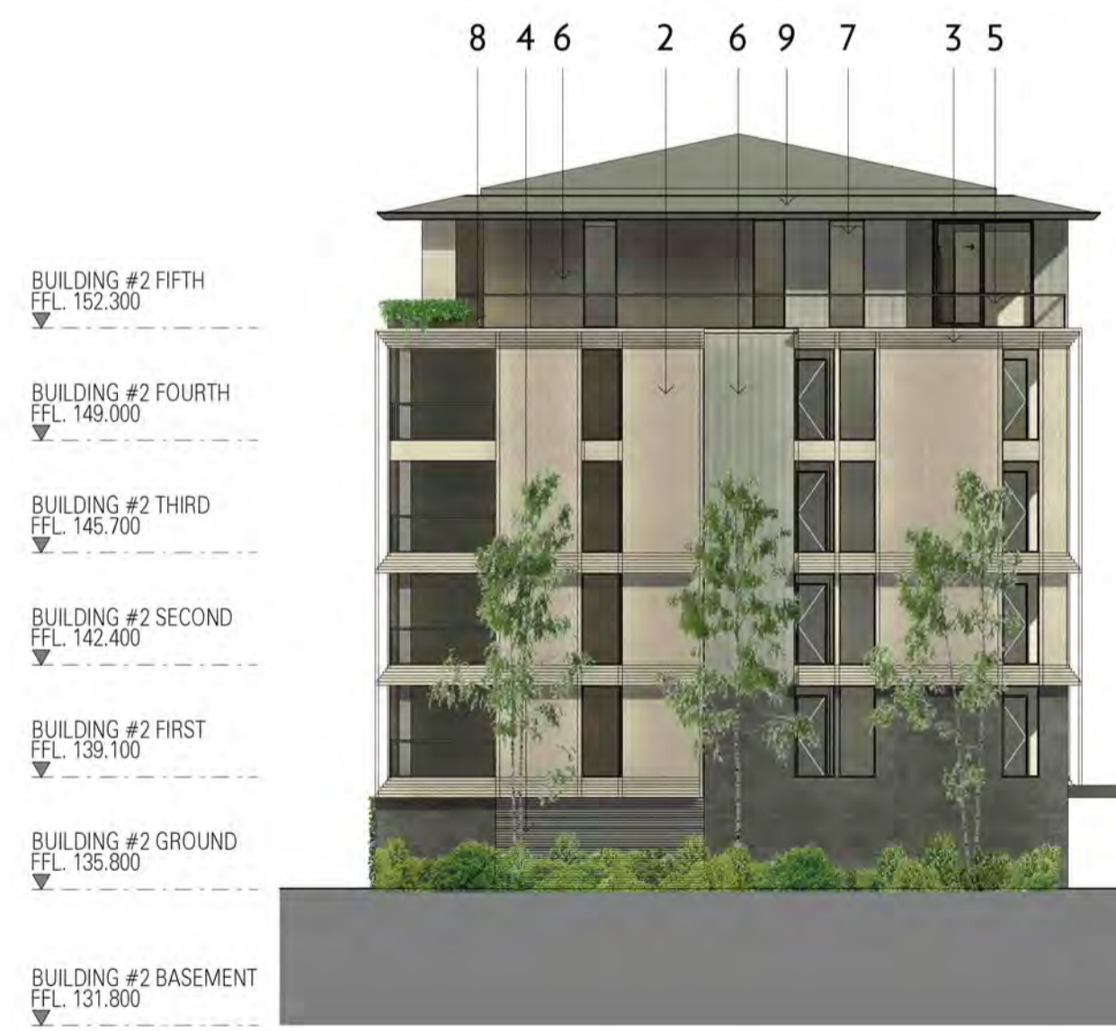
WEST ELEVATION - BUILDING 02 1:200
