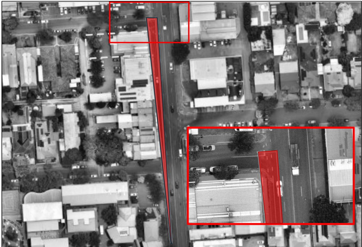
Figure 1 Sight Distance Envelope (South) – 2 Sec Reaction Time, 70km/h Design Speed – SISD: 151 Metres
