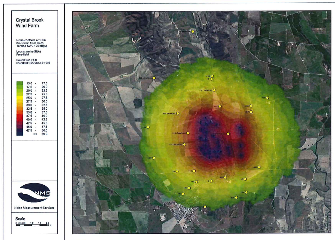
Plate 3: Calculations with 6m/s wind from the south, turbines at 105 dB(A) sound power level
