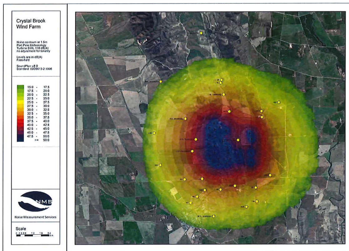
Plate 5: Calculations with Port Pirie wind rose data, turbines at 110 dB(A) sound power level
