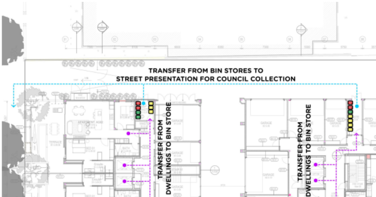
Figure 5-15 Bin storage arrangements and transfer paths
