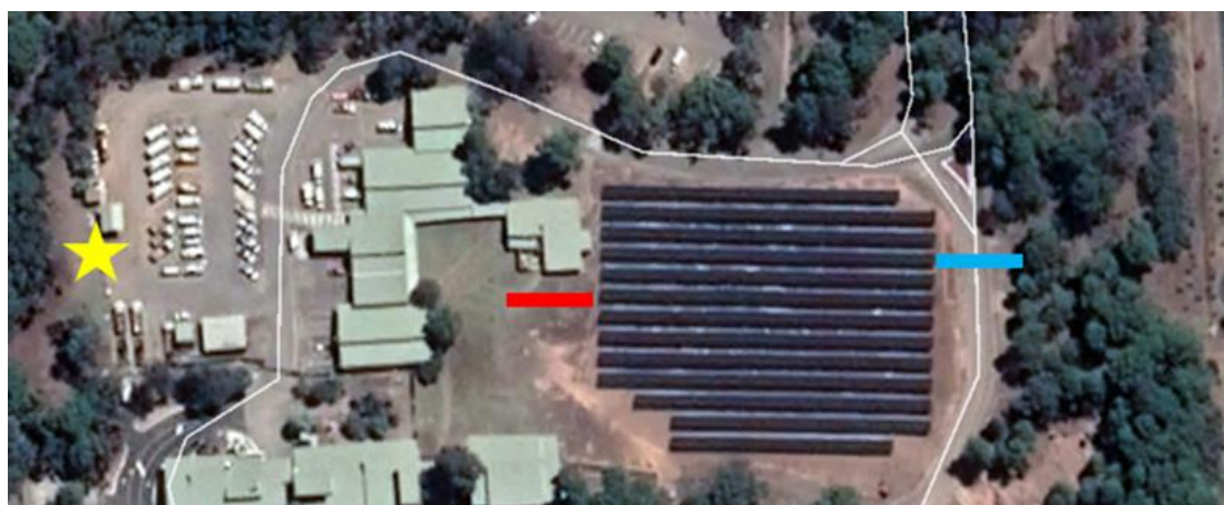
Figure 6 - Site aerial view showing the array, locations of temperature measurements (red and blue lines) and the temperature control location (star).
