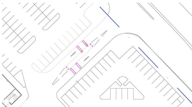
Figure 15: Left-in/left-out movements with single entry and exit gates at access 10
