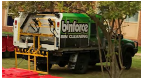
Figure 5-8 On-site bin wash system for rear-lift trucks on back of ute. Source: http://binforce.com.au/
