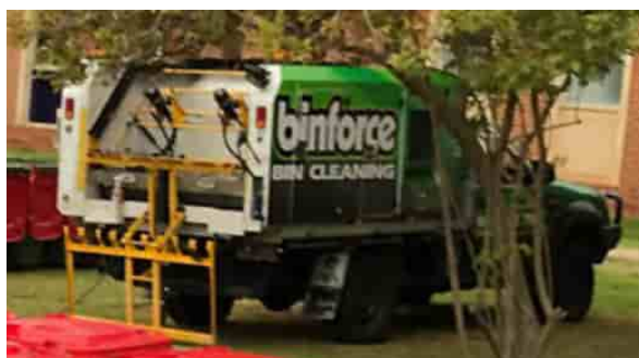
Figure 4-6: On-site bin wash system for rear-lift trucks on back of ute. Source: http://binforce.com.au/
