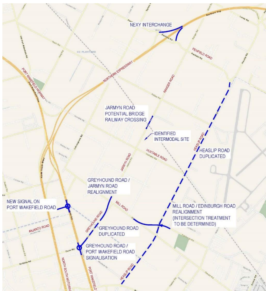
Figure 4: Potential Infrastructure Treatments
