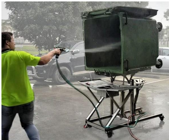
Figure 5-6 Mechanical bin washer Source: https://emoveit.com.au/product/bin-blaster-mobile-wheelie-bin-washer
