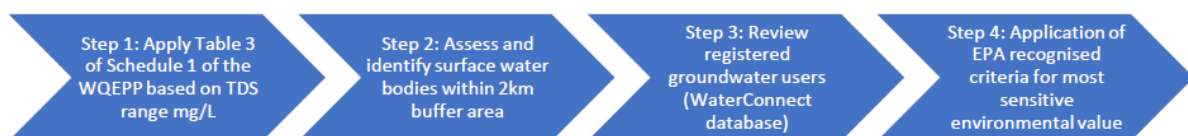
Figure 3-1 Process to Determine Environmental Values of Groundwater at a Site
