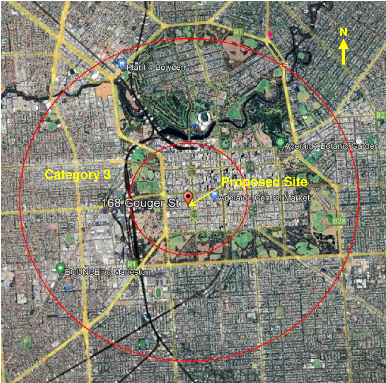
Figure 3: Assumed terrain categories for wind speed estimation.
